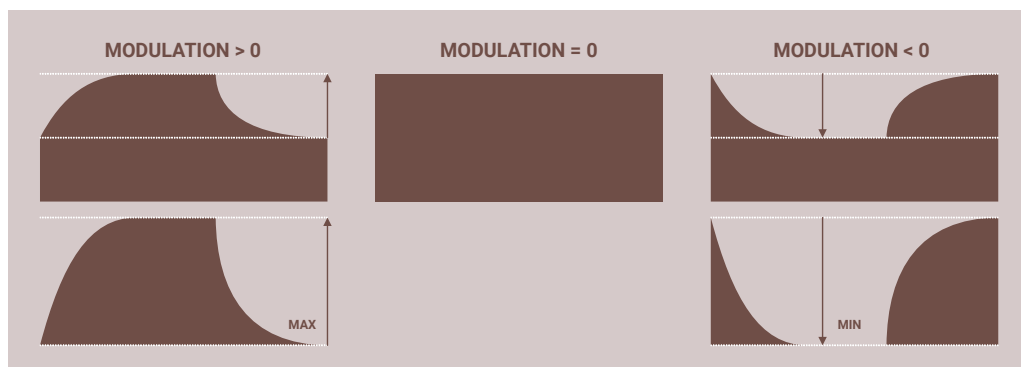
A diagram showing how different envelope modulation values affect amplitude
