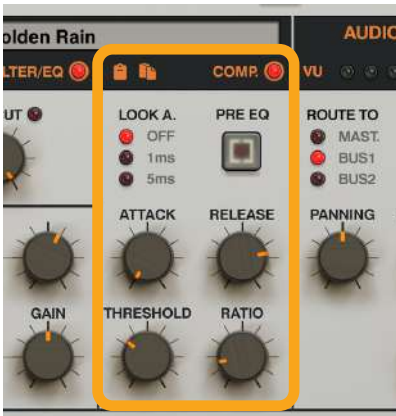
The Compressor section
